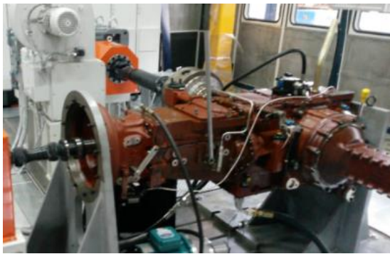
Figure 1. Sample gearbox bench testing
