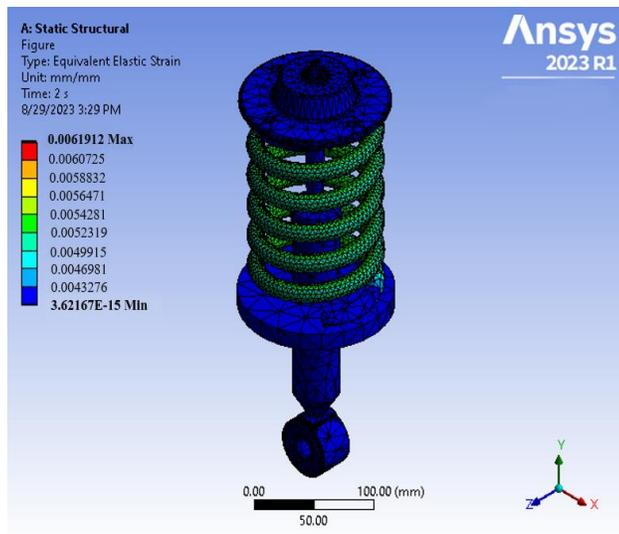
Figure 17. Shock absorber equivalent elastic strain profile for alloy steel wire (A231)
