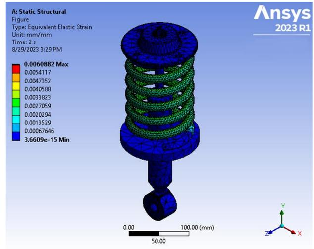
Figure 18. Shock absorber equivalent elastic strain profile for stainless steel wire (A313)
