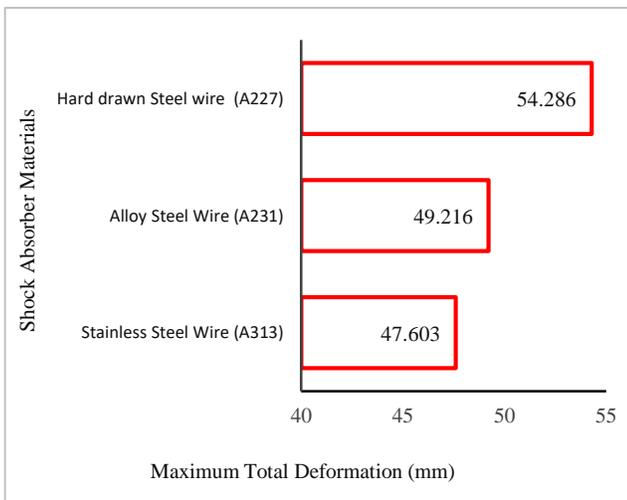
Figure 7. Plot of maximum total deformations for the three shock absorber materials
