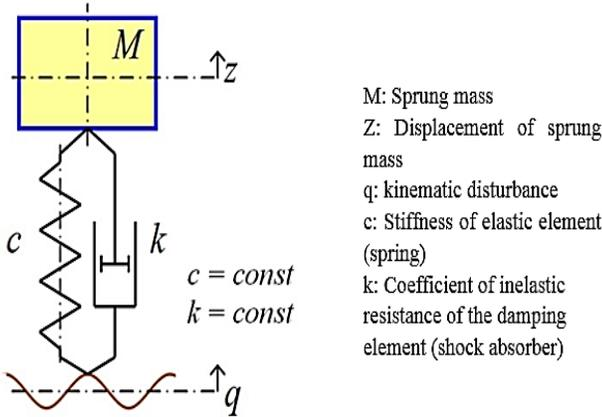
Figure 1. Linear vibrating system with damping characteristics
