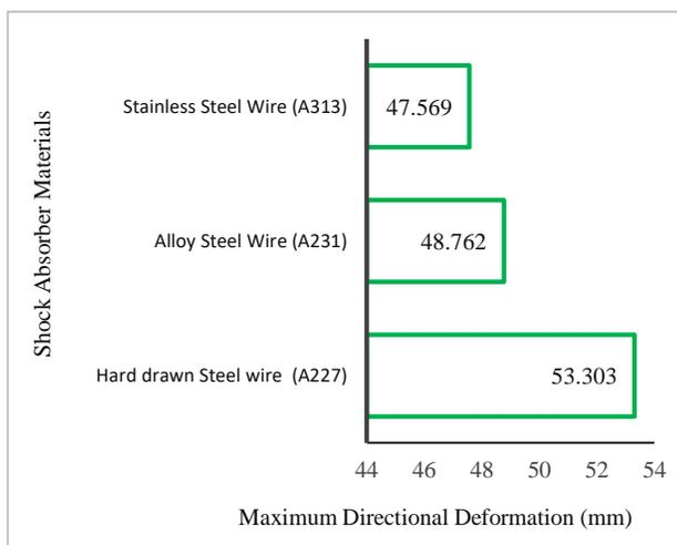
Figure 11. Maximum directional deformations for the three shock absorber materials
