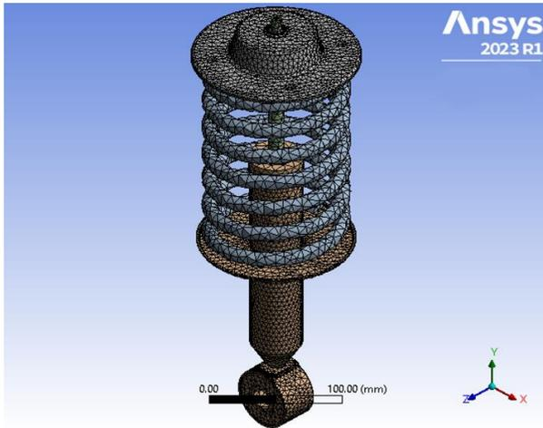
Figure 3. Mesh visualization of the shock absorber model
