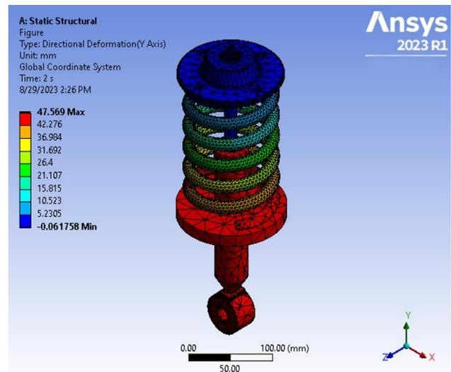
Figure 8. Shock absorber directional deformation profile for stainless steel wire (A313)
