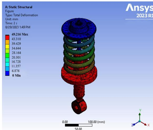
Figure 5. Shock absorber total deformation profile for alloy steel wire (A213)
