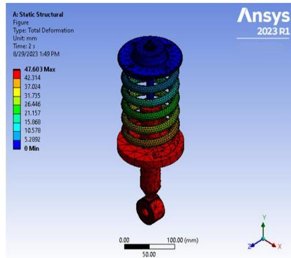
Figure 4. Shock absorber total deformation profile for stainless steel wire (A313)
