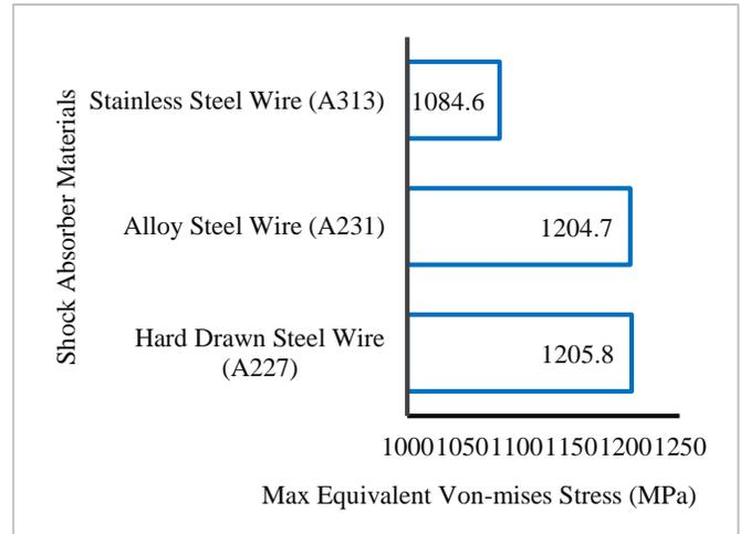
Figure 15. Plot of maximum equivalent von-mises stress for the three shock absorber materials
