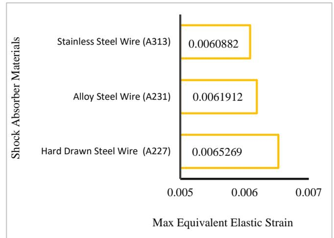
Figure 19. Plot of maximum equivalent strain for the three shock absorber materials
