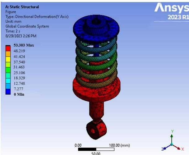
Figure 10. Shock absorber directional deformation profile for hard drawn spring wire (A227)
