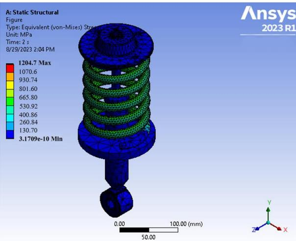
Figure 13. Shock absorber equivalent von-mises stress profile for alloy steel wire (A231)
