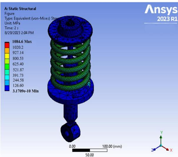
Figure 14. Shock absorber equivalent von-mises stress profile for stainless steel wire (A313)
