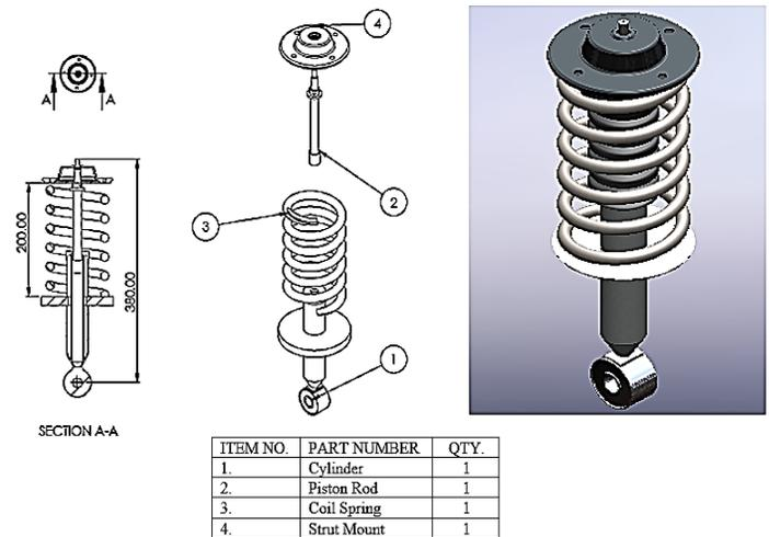
Figure 2. Shock absorber assembly
