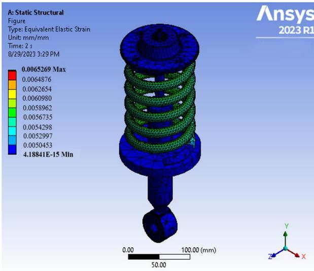
Figure 16. Shock absorber equivalent elastic strain profile for hard drawn spring wire (A227)
