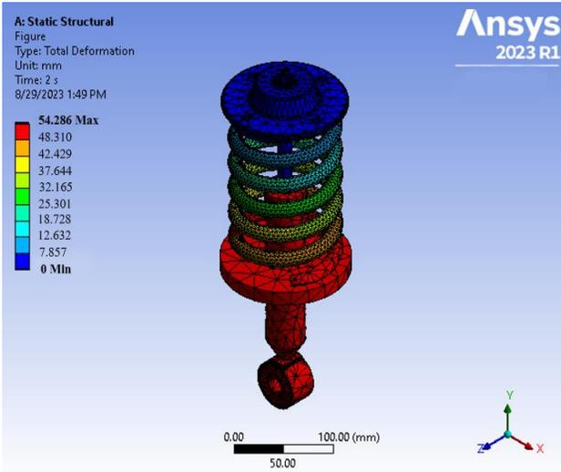
Figure 6. Shock absorber total deformation profile for hard drawn spring wire (A227)
