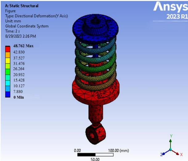
Figure 9. Shock absorber directional deformation profile for alloy steel wire (A231)
