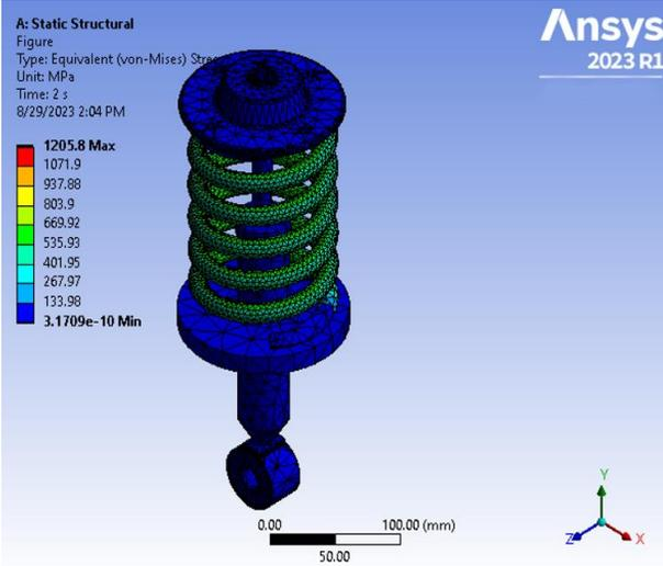
Figure 12. Shock absorber equivalent von-mises stress profile for hard drawn spring wire (A227)
