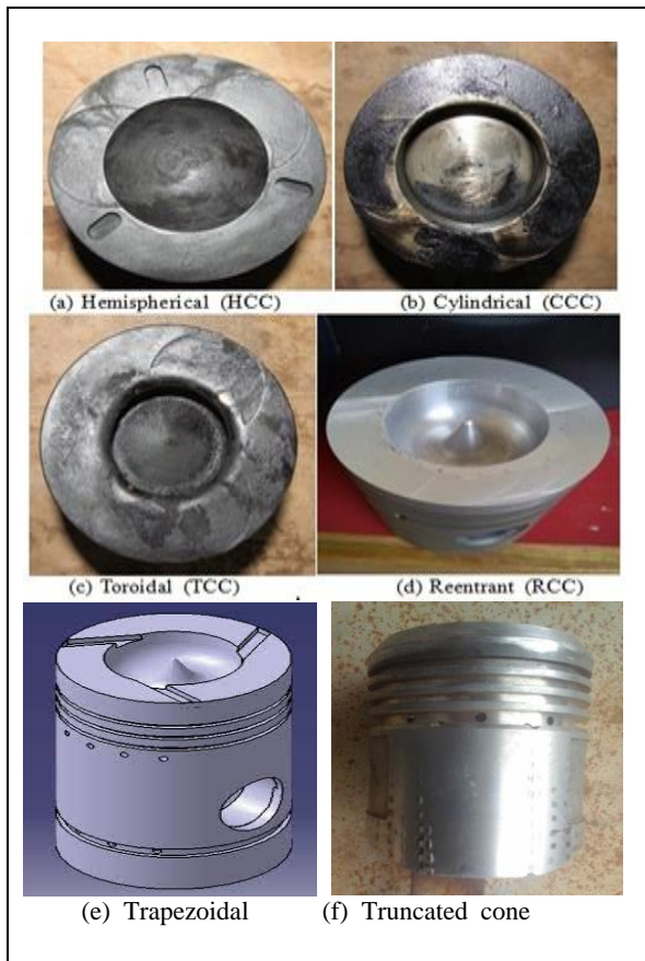
Figure 1. Selected piston bowl geometry
