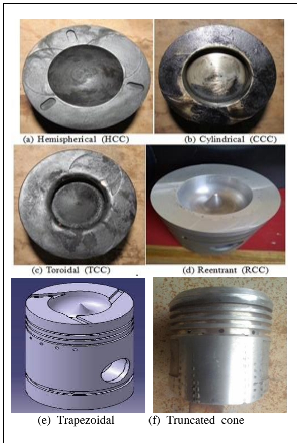
Figure 1. Selected piston bowl geometry
