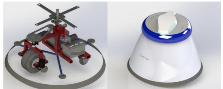
Figure 1. General view of the chassis and designed autonomous robot for the feed pushing
