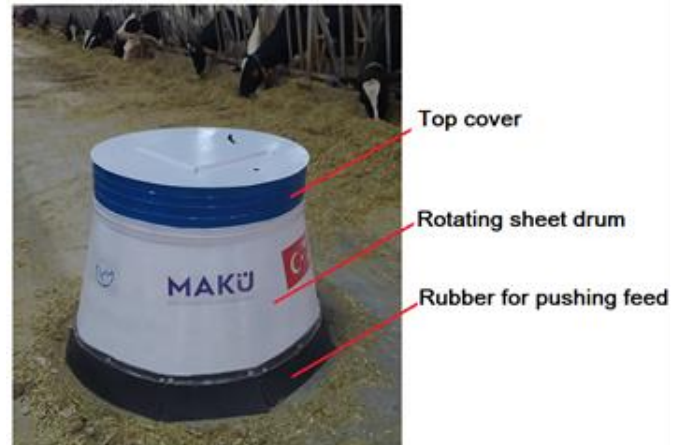
Figure 8. Manufactured feed pushing robot
