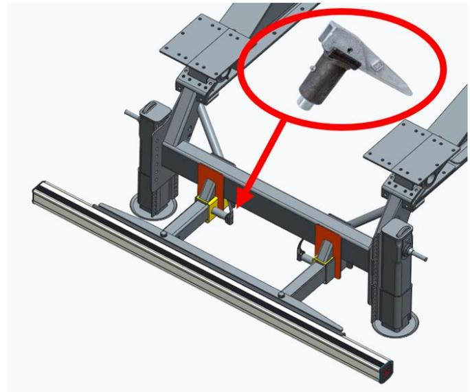
Figure 13. Design revision: Additional support brackets
