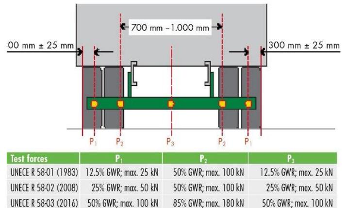
Figure 3. Test loads of UNECE R58.03 [4]
