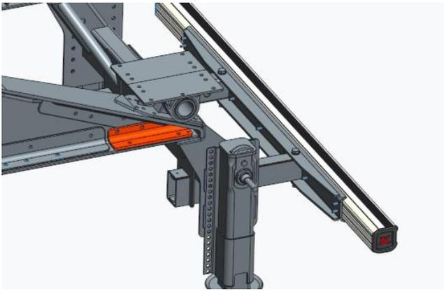
Figure 7. Design revision: Additional L support bracket
