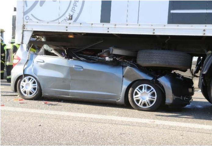
Figure 1. Typical rear underrun collision
