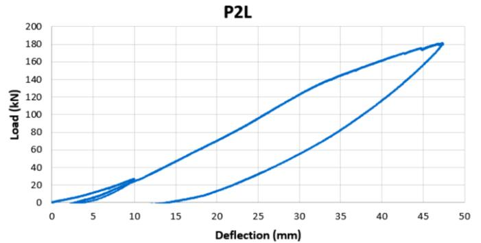
Figure 16. Deflection on P2 LEFT test case in second test
