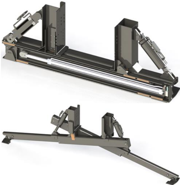
Figure 3. Closed and open position solid model of cross-type outriggers
