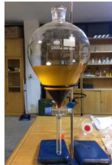
Figure 3. Separating glycerin in biodiesel
