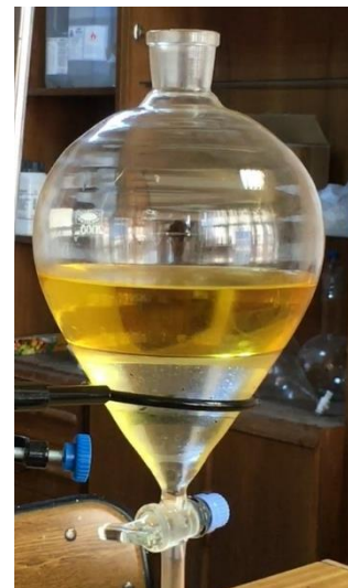
Figure 4. Biodiesel fuel washing process
