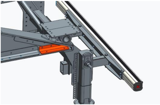
Figure 7. Design revision: Additional L support bracket
