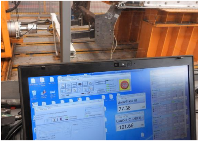
Figure 19. Photo of deflection on P3 MIDDLE test case in second test
