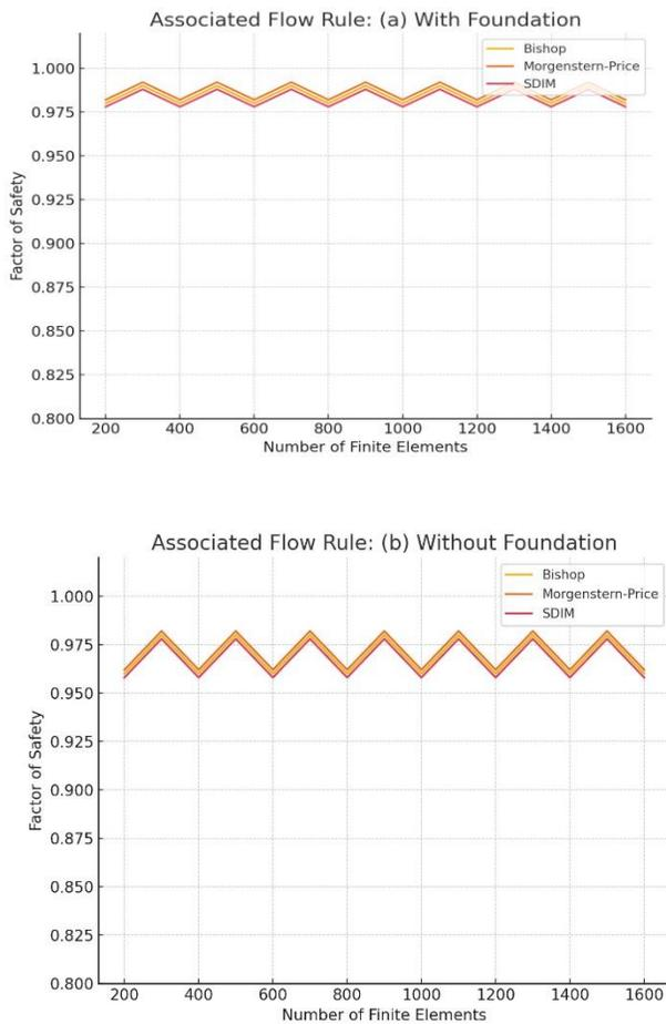
Figure 7. Comparison of factor of safety versus the number of finite elements for the associated flow rule. (a) With foundation and (b) without foundation. (Parameters:  $\gamma = 20 \text{ KN/m}^2$ ,  $\phi = 19.6^\circ$ ,  $c = 3 \text{ KPa}$ , Poisson ratio = 0.33,  $E = 100000 \text{ KN/m}^2$ ,  $\psi = 19.6^\circ$ )
