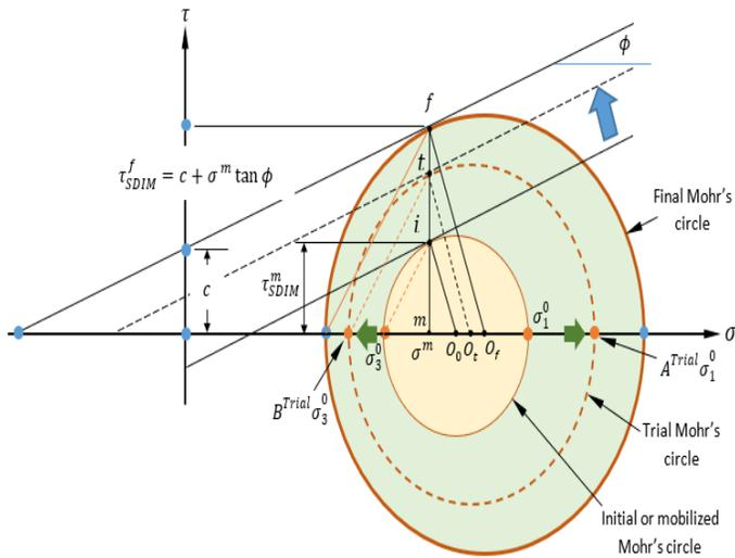
Figure 3. Evolution of principal stresses in the Stress Deviator Increasing Method (SDIM)[18].
