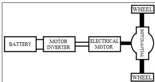
Figure 10. Schematic Of A Direct Drive Electrical Vehicle
