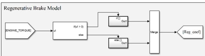
Figure 12. Regenerative Brake Model
