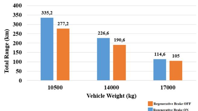
Figure 22. Effect of Regenerative Braking Gain on Total Range
