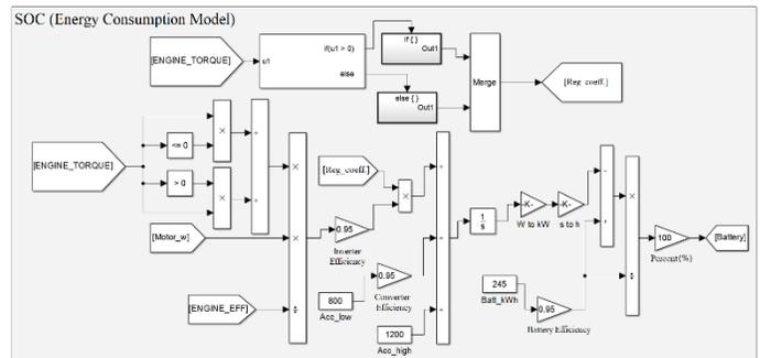
Figure 13. "State of Charge" Energy Consumption Model
