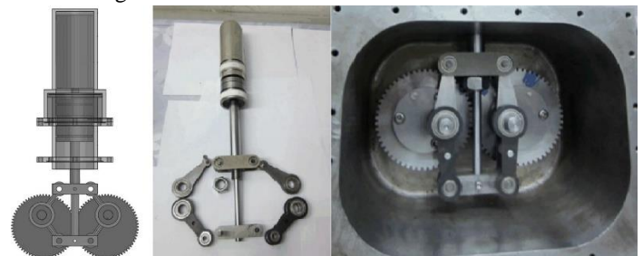
Figure 19. β-type Stirling engine with rhombic drive mechanism [59,60]
