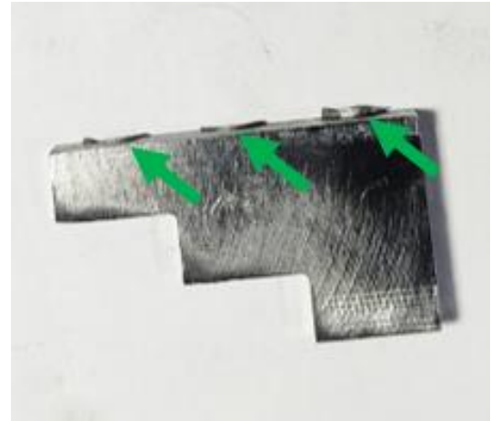
Figure 9. Hole burr formation due to hole length when tool run-out is present before maintenance
