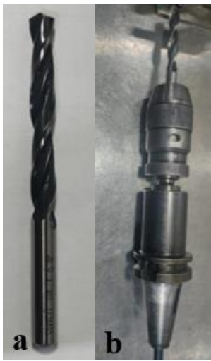
Figure 5. (a) HSS drill Ø 9.8 mm (b) Ball holder and drill
