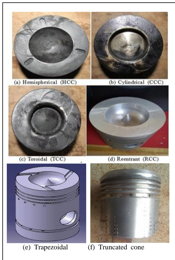
Figure 1. Selected piston bowl geometry
